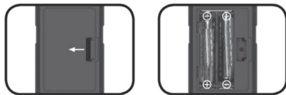
Open the battery cover on the back of the unit and insert the batteries, observing the correct polarity, and close the cover. Use AAA 1.5V batteries.
