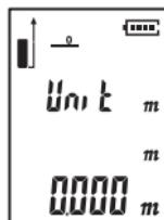
In the unit setting state, briefly press the button to change the unit of measurement.
