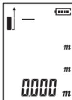
In measurement mode, press and hold the button for 2 seconds to enter continuous measurement mode.
