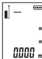
In measurement mode, short press the button , and the instrument will emit the laser, point at the object whose distance is to be measured, and short press the button again for single distance measurement.The measurement result is shown in the main display area. Subsequent measurements scroll across the secondary display up to a total of 3.
