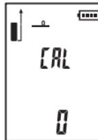
To ensure the accuracy of the instrument, a calibration function is provided. In the calibration function: press the button briefly to adjust the calibration value.
